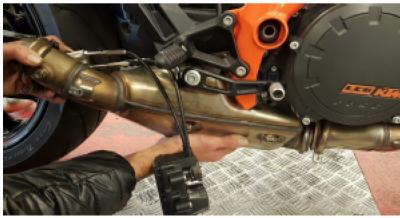
(d) Remove trains and the plate of the actuator. To do so please secure
