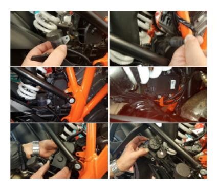
(c) To facilitate movement of the original silencer we recommend a lightweight preloading to the rear spring by either an assistant or a strap.
