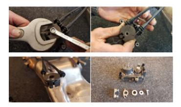
Install the BODIS stop in the subsequent order, and tighten.
